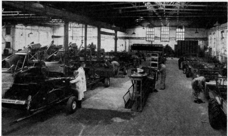
Combine harvesters, pick-up balers and manure spreaders being assembled at the Albion Works
