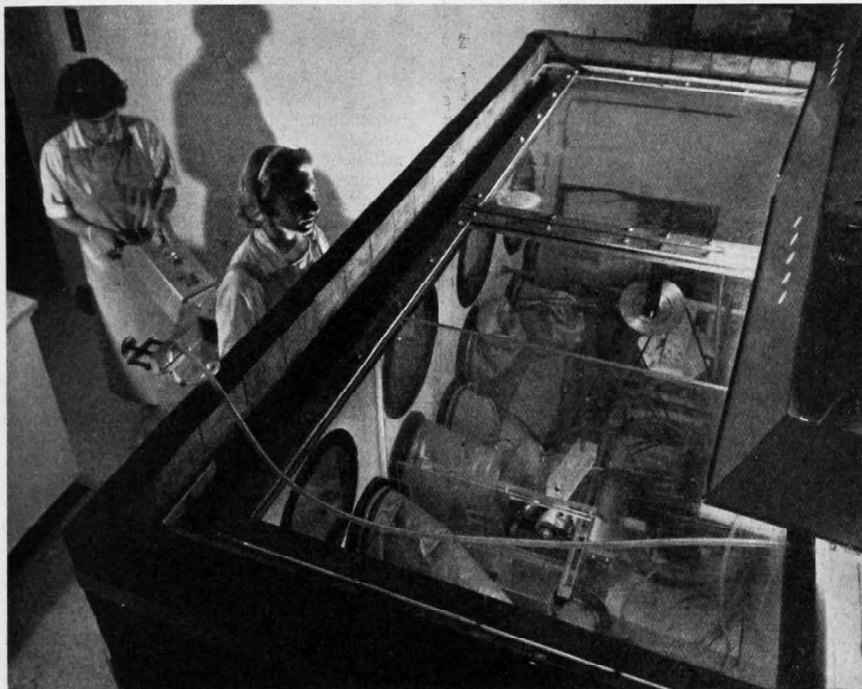
A remotely controlled miniature machine shop at the Radiochemical Centre, Amersham. New buildings have been completed, at a cost of £200,000, housing equipment and administrative services to cope with the greatly increased world-wide demand for radiochemicals
