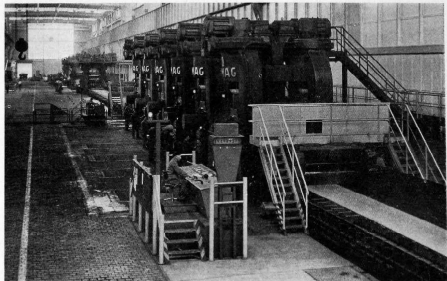
Fig. 3—The 66in hot continuous strip mill. In the foreground are the six finishing stands
